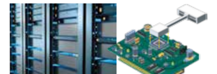
A small, high-performance two-phase cooler (Siphorex), developed for cooling CPUs of servers at data centers
