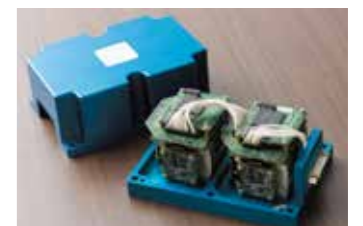
The MEMS gyroscope consists of two units as one set, each checking the other for abnormalities to prevent any radiation incidents in space.
