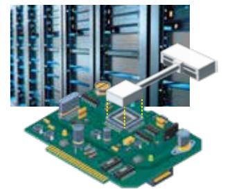
A small, high-performance two-phase cooler (Siphorex), developed for cooling CPUs of servers at data centers
