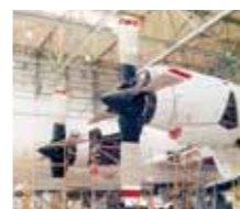
P-3C propeller system Driven by an engine to produce thrust
