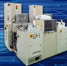
PECVD equipment for oxidized film/nitride film
