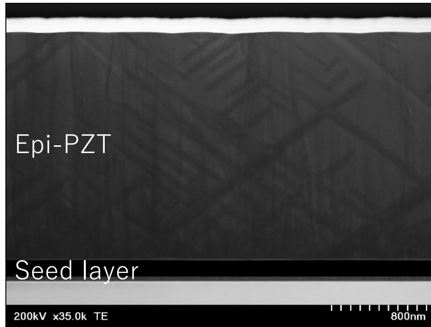
Cross Section of Epi-PZT film
