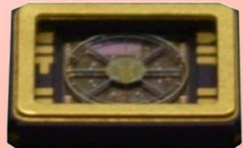
Piezoelectric MEMS gyro CRM series oscillator
